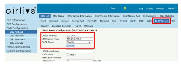
The setup is now complete and the PC connected to the ONU will get an IP address from the Router in front of the OLT.
