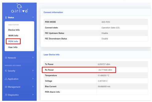
If ONU RX power shows '-inf' after fiber plug-in, please replace PON module and/or replace a with another ONU to check.
