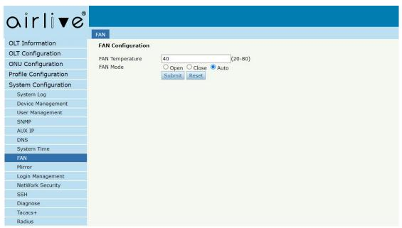
(2) Listen if there is any noise coming from the fan inside the OLT. Note the fan will not run if the OLT temperature is below the set FAN Temperature.
